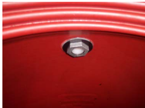
An adaptor secured by silicone, washer, and locknut
