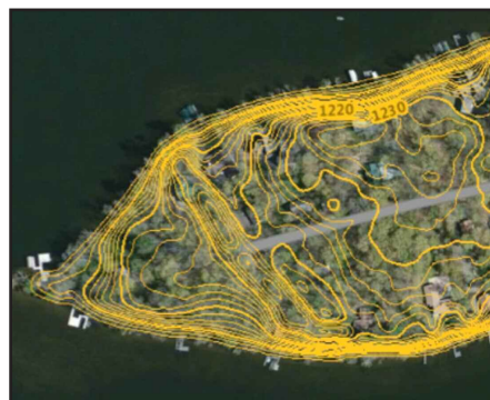
A peninsula of Gull Lake showing two foot contour lines on an aerial image.
