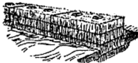
Figure 3: Constructing a straw bale barrier to slow runoff and prevent erosion.
