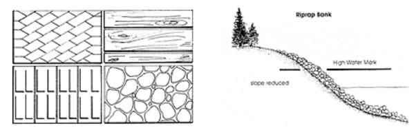
Rip rapping a shoreline with stones can be a good means of controlling erosion. It will likely require a permit from the DNR, so check with the local office before undertaking any actions. Although there are general guides to constructing rip rap, the specific circumstances of your case are vital to determining what should or can be done. Consult the DNR and the Soil and Water Conservation District for advice.
